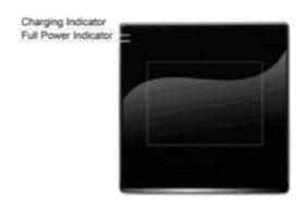
Charging Indicator: Red light represents charging the tablet. Full Power Indicator: Green light represents full battery power. The battery cannot be detected or malfunctioned when the Power-on Indicator and Charging Indicator are blinking; please check whether the battey is secured in the compartment and is in good condition. The battery is fully charged when Charging Indicator and Full power Indicator are on at the same time.
