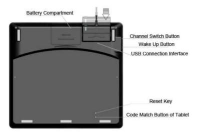
Battery compartment: A compartment stores tablet battery.
