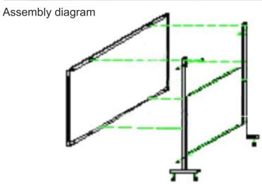
12. Hang the board to the four bolts position and fix the bolts tightly.
