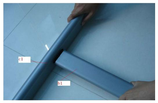
2. Connect beam b1 and vertical pole c2
